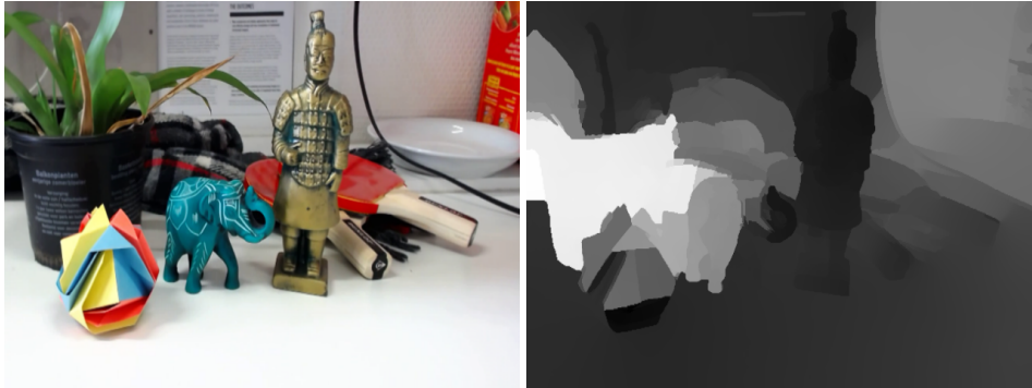
Figure 8. Example frame and initial two-view depth estimate for a manually recorded sequence. The initial image as well as its rectified version (using this depth estimate as input) are visible in Figure 9a.
