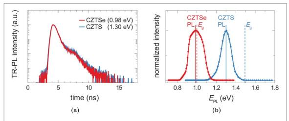
**Figure 3.** (a) Comparison of the PL decay obtained for both materials and, (b) comparison between PL main emission and  $E_g$  for CZTSe and CZTS. Reproduced with permission from [2] John Wiley & Sons. (© 2014 WILEY-VCH Verlag GmbH & Co. KGaA, Weinheim).
