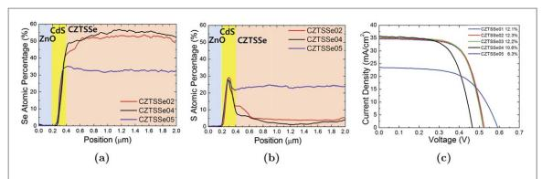
Figure 7. Selenium (a) and sulfur (b) depth profiles obtained using STEM-EDS measurements in CZTSSe absorber layers grown by chalcogenization with different  $SeS_2/Se$  chalcogen sources weight ratios. (c) Current density-voltage characteristics of the corresponding CZTSSe solar cells. Reproduced from [4] with permission of The Royal Society of Chemistry.
