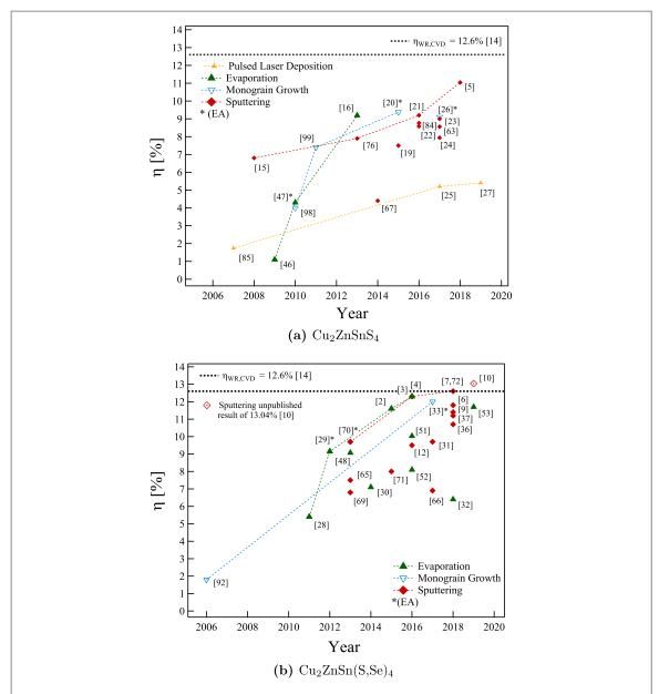
**Figure 1.** Evolution of the maximum efficiency  $\eta_{\text{max}}$  [%] for (a) CZTS-based and (b) CZT(S,Se)-based cells over the period of 2006–2019. In figure legend WR stands for world record and EA stands for effective area.
