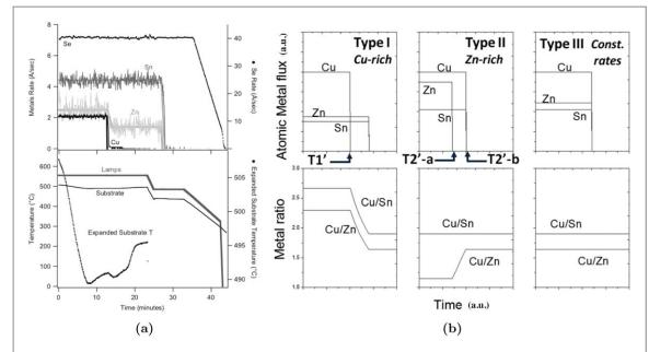
**Figure 2.** (a) Deposition data of the process for co-evaporated CZTSe materials reported by Repins *et al* [29]. Reprinted from [29], Copyright (2012), with permission from Elsevier. (b) Different composition regimes for co-evaporated CZTSe including Cu-rich, Zn-rich and constant rates by Hsu *et al* [48]. Reproduced with permission from [48] John Wiley & Sons. (Copyright © 2013 John Wiley & Sons, Ltd.).
