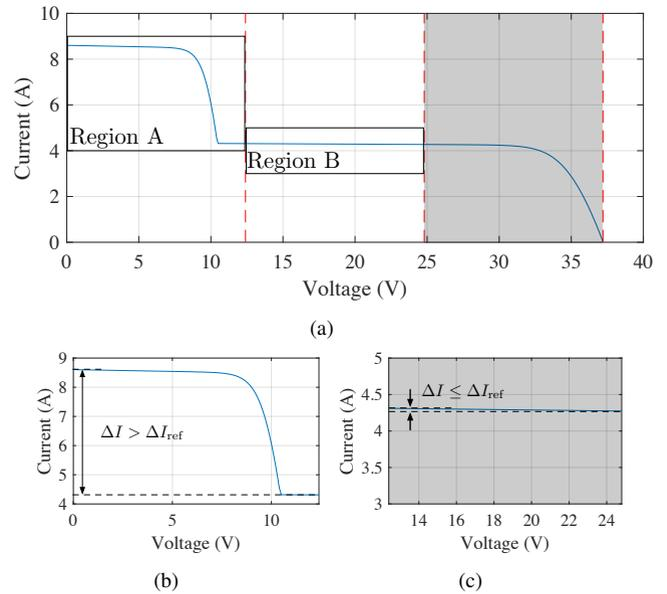
**FIGURE 3.** Initial selection rule for the Tabu List: (a) overall I-V curve; (b) region A; (c) region B.
