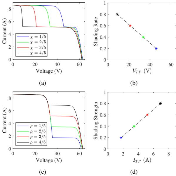
**FIGURE 5.** Relationships between the shading information and the position of the turning point for a PV string with five PV modules. (a) I-V curves with different shading rate information; (b) the relationship between the shading rate information and the voltage at the turning point  $V_{TP}$ ; (c) I-V curves with different shading strength information; (d) the relationship between the shading strength information and the current at the turning point  $I_{TP}$ .
