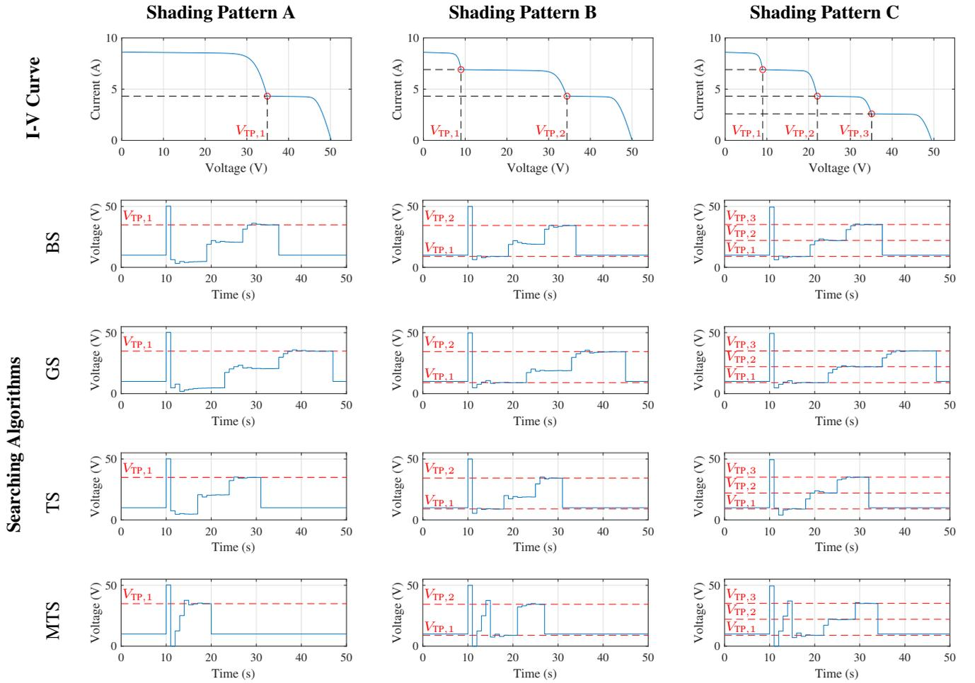
**FIGURE 6.** Comparison in the tracking traces from different searching algorithms under varied shading patterns (shading pattern A: {500,1000,1000,1000}W/m<sup>2</sup>, 25°C; shading pattern B: {500,800,800,1000}W/m<sup>2</sup>, 25°C; shading pattern C: {500,800,300,1000}W/m<sup>2</sup>, 25°C.).
