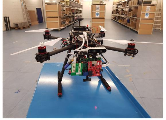
Fig. 2. Our NXP HoverGames drone with a 79 GHz Texas Instruments radar and an on-board camera.
