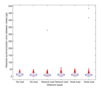
Fig. 8. Impact of the network and node load on the synchronization error.
