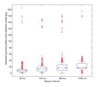
Fig. 7. Impact of the beacon interval on the synchronization error statistics.
