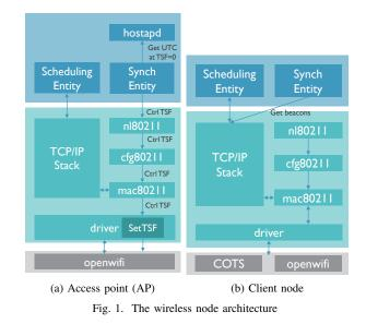
on the TSF counter received on the last beacon from the AP. Such synchronization is used only by the WiFi cards themselves to correctly calculate the time, like e.g. when the network allocation vector (NAV) time ends. Consequently, such synchronization is unaware of the time in the host itself and does not change the host time itself.
