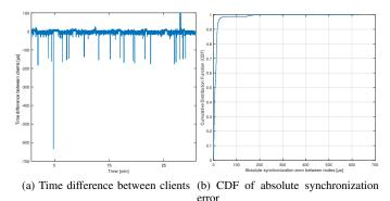
Fig. 5. Synchronization error between clients when TSF is controlled by PTP
