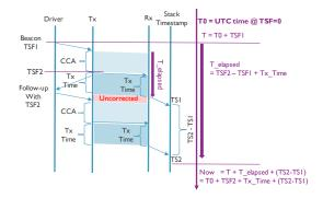
Fig. 2. Synchronization mechanism time diagram
