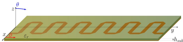
FIGURE 2 3-D view of the rampart line antenna and adopted reference system
