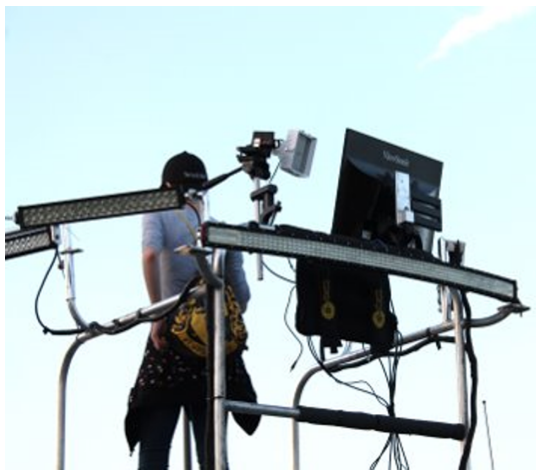
Fig. 9. NIR camera system mounted on the top of a vehicle.
