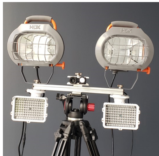
Fig. 2. Mounted Vis and NIR cameras and illumination. Halogen lamps are mounted above the cameras, and NIR LED illuminators are mounted below.
