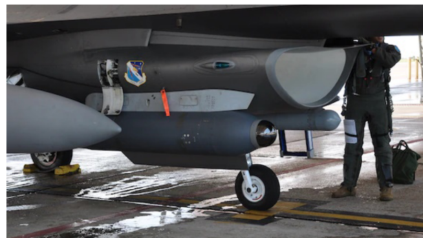
Fig. 1. Air Force F-16 Legion Pod IRST [3]. Similar sensors are embedded on the SAAB Gripen, the Eurofighter Typhoon, and Dassault’s Rafale.
