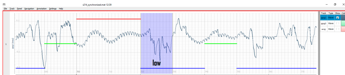
Figure 5. Example PPG signal in epoch mode: blue, green, and red color bars stand for different signal quality levels assigned to 10 s segments.
