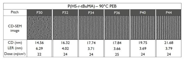
Figure 9. Patterning performance of the P(HS-r-tBuMA) polymer-based resist at 90 °C PEB.
