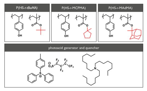
**Figure 1.** The chemical structure of the poly(hydroxystyrene-*ran*-tert-butyl methacrylate) (P(HS-*r*-*t*BuMA)), poly(hydroxystyrene-*ran*-1-methylcyclopentyl methacrylate) (P(HS-*r*-MCPMA)), and poly(hydroxystyrene-*ran*-1-methyladamantyl methacrylate) (P(HS-*r*-MAdMA)) polymers, and associated photoacid generator ((4-methylphenyl)diphenylsulfonium nonaflate) and quencher (trioctylamine) used in the full resist formulation.
