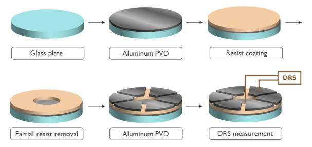
**Figure 2.** Schematic representation of a sample preparation for a dielectric response spectroscopy (DRS) measurement of a resist layer.
