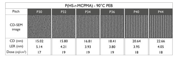
**Figure 8.** Patterning performance of the P(HS-*r*-MCPMA) polymer-based resist at 90 °C post-exposure bake (PEB).
