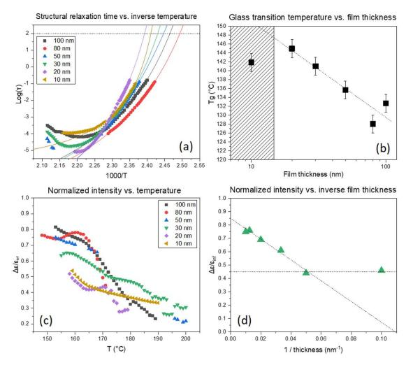
Figure 4. (a) The determined  $T_g$  values for each thickness; (b) the normalized intensity versus temperature; (c) and the normalized intensity versus the inverse film thickness (d).
