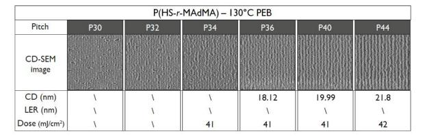
Figure 13. Patterning performance of the P(HS-r-MAdMA) polymer-based resist at 130 °C PEB.
