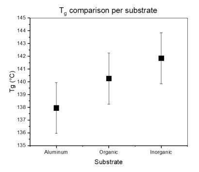
Figure 7. Comparison of  $T_{\rm g}$  values on the different underlayers.
