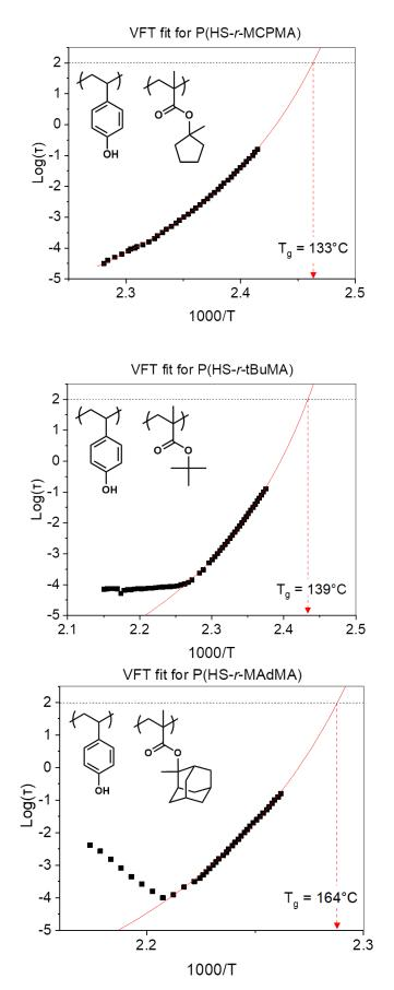
**Figure 3.** Logarithmic structural relaxation time versus the inverse of temperature plots for the different 30 nm thin film polymer samples.
