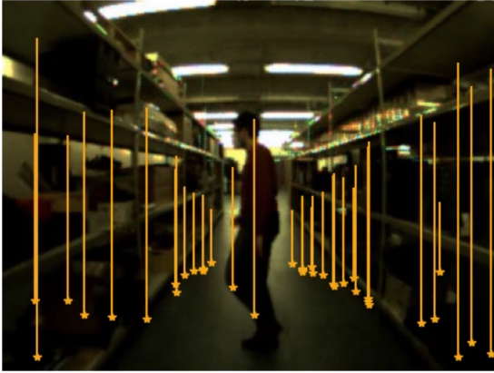
Fig. 4: Radar columns obtained by projecting the range-azimuth radar detections on the image plane by homography (star-shaped markers) and extending them in height to cover their spatial context.
