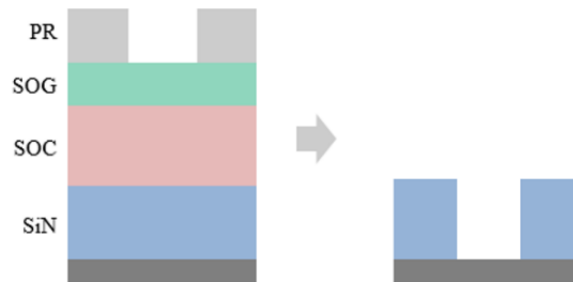
Figure 4: Stack at the inspection steps (left) ADI and (right) SiN open
