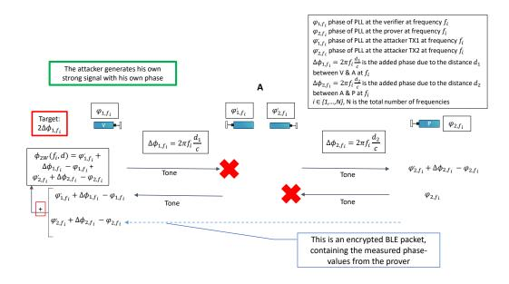
Figure 11: Phase manipulation attack on the MCPD.
