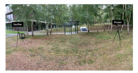
Figure 13: Outdoor wireless measurement setup.
