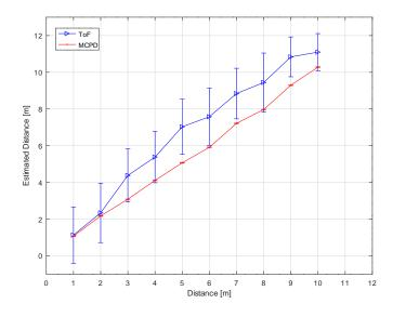
Figure 14: Outdoor distance measurement results.
