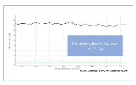
Figure 20: MCPD- and ToF-based distance measurements under relay attack.
