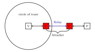
Figure 7: Relay attack on a distance bounding protocol.
