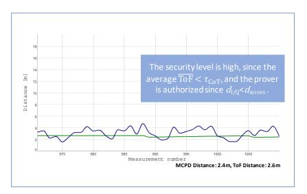
**Figure 17:** MCPD- and ToF-based distance measurements when the prover is close to the verifier.
