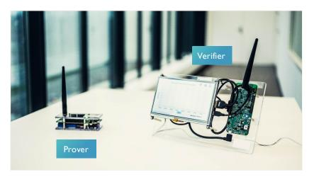
Figure 12: The proposed SDB solution is implemented on NXP KW36 chips.
