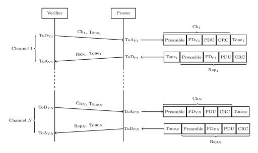
Figure 4: The distance bounding (or ranging) stage of our protocol.
