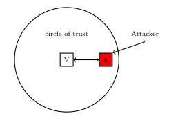
**Figure 6:** Impersonation attack. Note that there is no prover present in this attack, and that the attacker could also be outside the circle of trust.
