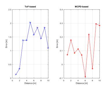
Figure 16: Error in ToF-based and MCPD-based distance measurements.
