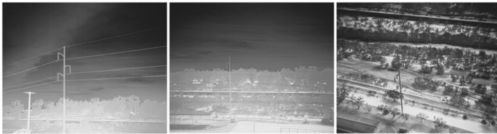
Fig. 1. Power Lines in the LWIR. Figure 1(a) (left) shows the wires against a cold sky where the ground reflection makes the wires bright. Figure 1(b) (middle) shows where the wire radiance matches the sky path radiance (i.e., no contrast). Figure 1(c) (right) shows a look down where the wires are dark reflecting cold sky against a warmer ground background.
