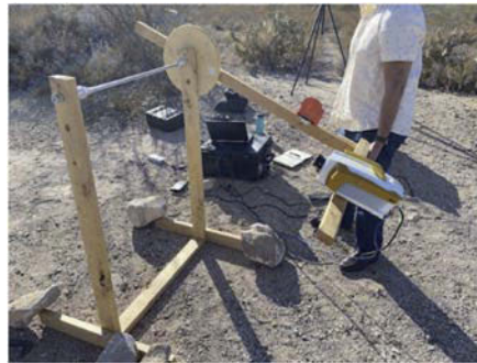
Fig. 4. Apparatus which holds the either the LWIR sensor or MWIR sensor (pictured) which contains the wire in the middle of the rotational axis, an arm holding a sensor at a constant distance, an inclinometer on the arm and a large disc to clamp the arm in place.
