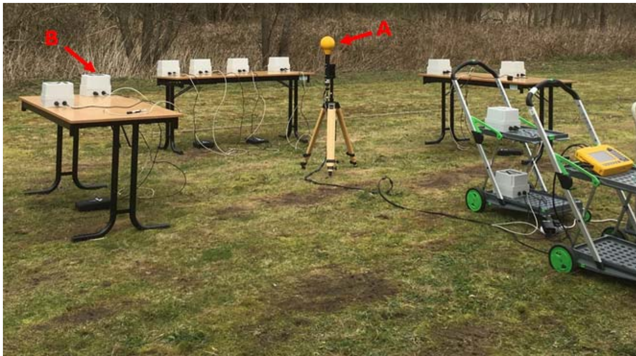
Figure 1. Setup of in-situ validation. A) NARDA SRM-3006, B) one of the ten EMF sensors. The probe of the SRM-3006 was installed on a height of 1.2m, the height of the tables is 0.8m.
