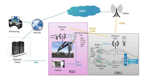
Figure 8 – Smart Highway Architecture
