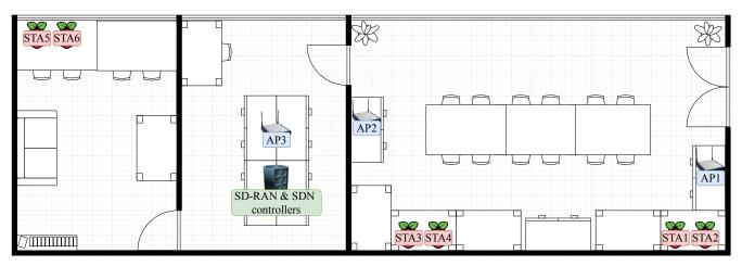
Figure 6. Testbed deployment scenario.
