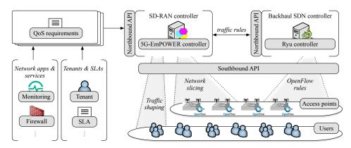
Figure 1. SDN-enabled layered network architecture.
