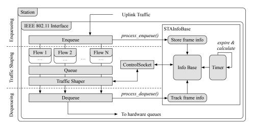
Figure 5. Traffic shaping in the simplified queue structure and data flow in an Station (STA).
