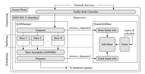
Figure 4. Queueing delay monitoring in the simplified queue structure and data flow in an AP.
