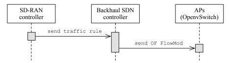
Figure 2. Sequence diagram of the traffic rule creation process.
