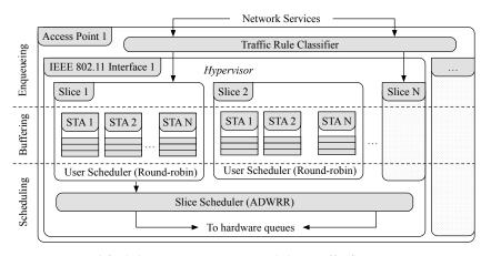
Figure 3. Simplified slice queue structure and data traffic flow in an Access Point (AP).
