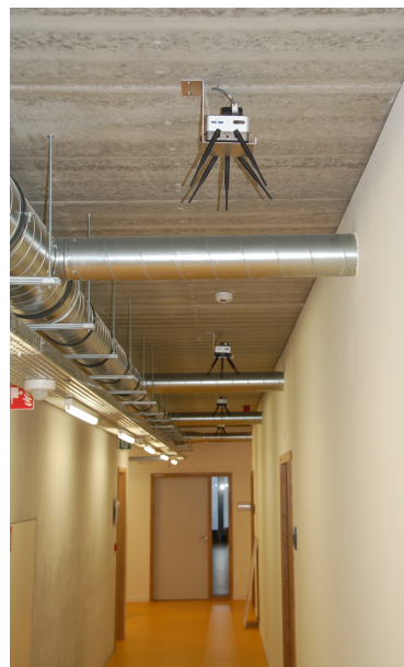
Figure 6. A subset of imec Wireless OfficeLab sensor nodes, deployed on the ceiling in an office environment spanning different floors of 805 m 2 , separated by reinforced concrete.
