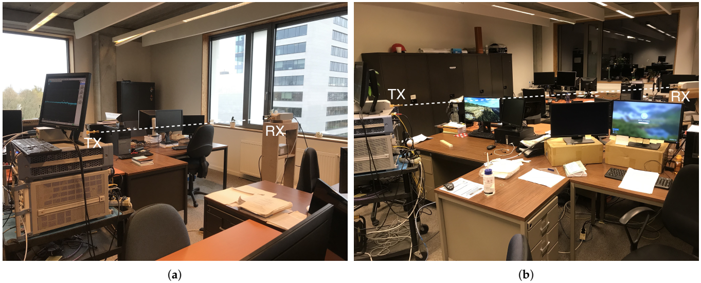
Figure 2. Line-of-Sight measurement tracks in office environment. (a) Track 1 with a distance of 2 m; (b) Track 2 with a distance of 2.9 m.
