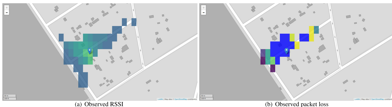
FIGURE 4. Observed RSSI and packet loss for IEEE 802.11n.
