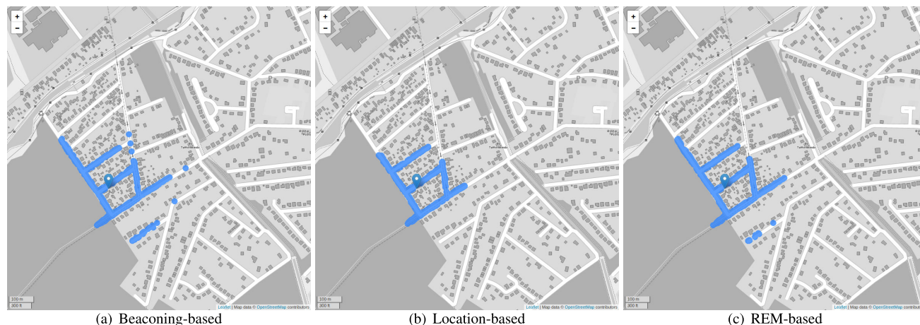
FIGURE 7. IEEE 802.11ah coverage achieved by different algorithms (95th percentile distance).
