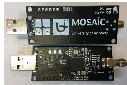
FIGURE 4. The USB transceiver that was utilized in the experiment.
