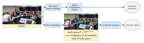
Figure 2. Data-processing pipeline for engagement estimation.
