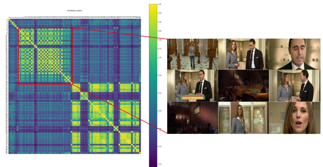
Figure 7. Estimated shot similarity for RAI video 23353. The figure also shows key frames of a selected LSU (red box).
