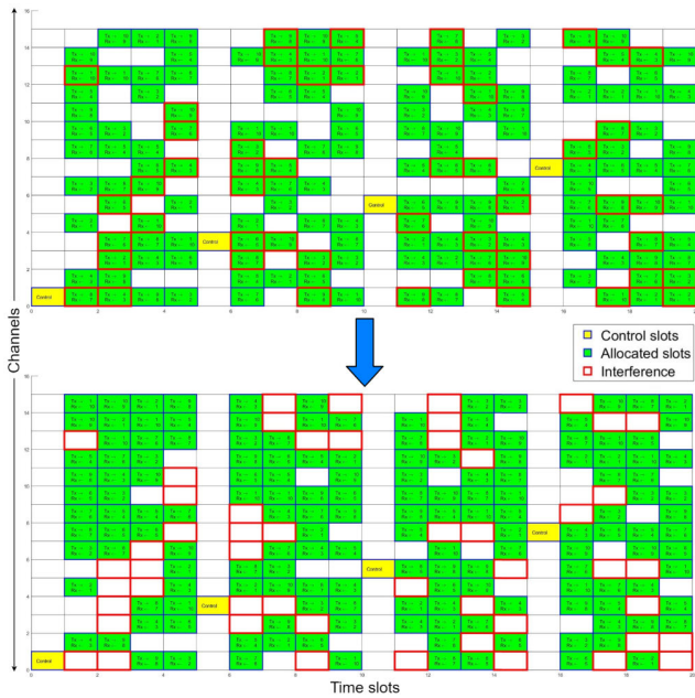
FIGURE 11. Superframe state of 10 nodes network before and after mitigation of external interference.
