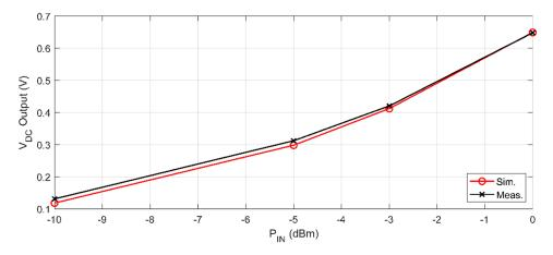
**Figure 7.** Textile rectifier output  $V_{DC}$  vs. input power  $P_{IN}$  (2.45 GHz).
