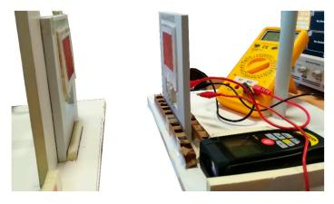
Figure 13. Single rectenna PCE measurement setup.
