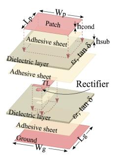
Figure 10. Perspective view of textile rectenna.
