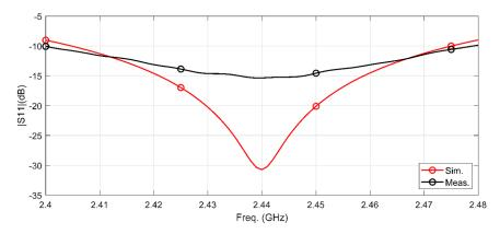
**Figure 2.** Electromagnetically coupled microstrip patch antenna's simulated and measured reflection coefficient in free-space.
