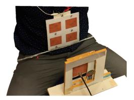
Figure 17. On-body measurement setup.
