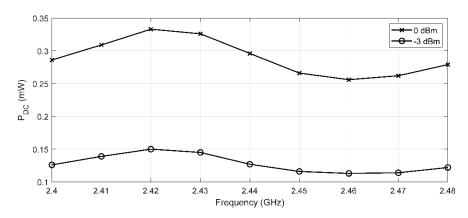
**Figure 8.** Textile rectifier output DC power  $P_{DC}$  vs. Frequency.
