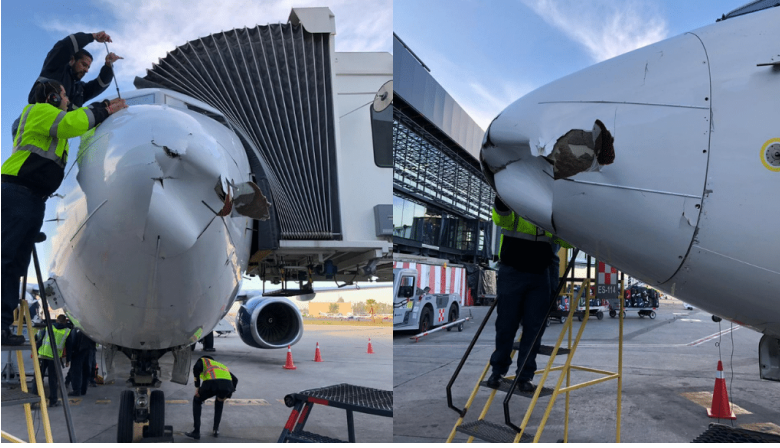
Figure 1.1 Nose cone and radome damage to an airplane on final approach to a Mexican airport caused by drone. [8]
