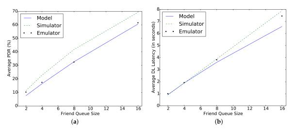
**Figure 8.** Comparing emulator, simulator, and model for different FQ at  $\mu_p = 1$  s,  $T_{PI} = 30$  s, C = 1 mF,  $P_h = 0.1$  mW,  $T_{AT} = 5$  ms. (a) Average packet delivery ratio; (b) DL latency.
