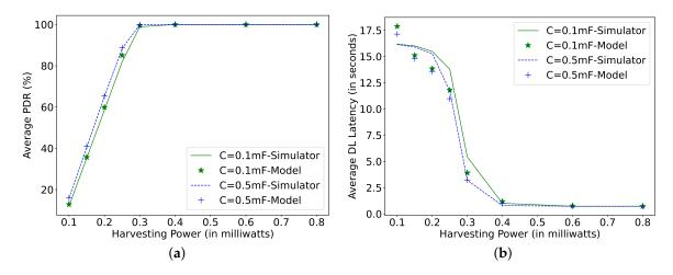
**Figure 9.** Comparing simulator and model for different harvesting powers at  $\mu_p = 1$  s,  $T_{PI} = 1$  s, N = 16,  $T_{AT} = 0$  ms. (a) Average packet delivery ratio; (b) DL latency.
