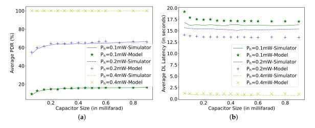
**Figure 10.** Comparing simulator and model for different capacitor sizes and harvesting power at  $\mu_p = 1$  s,  $T_{PI} = 1$  s, N = 16,  $T_{AT} = 0$  ms. (a) Average packet delivery ratio; (b) DL latency.
