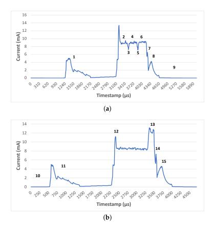
**Figure 5.** Current consumption of nRF52840 with the state number as defined in Table 1. (**a**) Current consumption during FP; (**b**) Current consumption during Scan.
