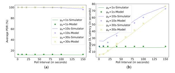
**Figure 11.** Comparing simulator and model for different Poll Intervals at C = 0.1 mF,  $P_h$  = 0.1 mW, N = 16,  $T_{AT}$  = 0 ms. (a) Average packet delivery ratio; (b) DL latency.
