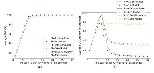
**Figure 14.** Comparing simulator and model for different packet arrival rate at C = 0.1 mF,  $P_h = 0.1 \text{ mW}$ , N = 16. (a) Average packet delivery ratio; (b) DL latency.
