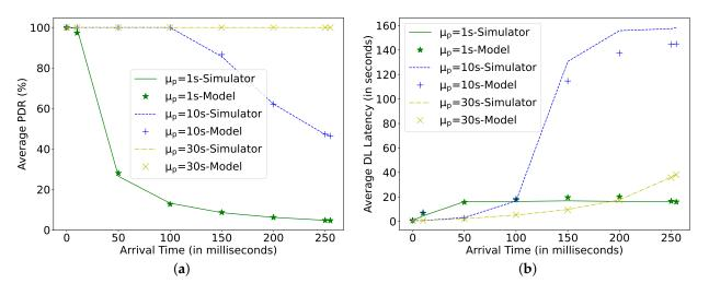
**Figure 13.** Comparing simulator and model for different arrival times (AT) at C = 4 mF,  $P_h = 1 \text{ mW}$ , N = 16,  $T_{PI} = 1 \text{ s.}$  (a) Average packet delivery ratio; (b) DL latency.
