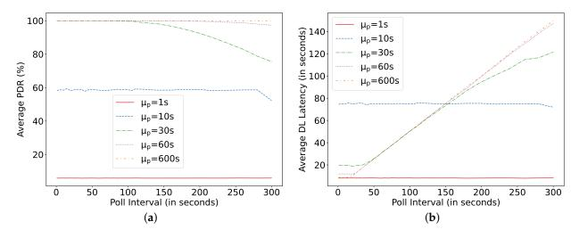
**Figure 16.** Asset monitoring at C = 5 mF,  $P_h$  = 0.1 mW, N = 8,  $T_{AT}$  = 5 ms for different packet arrival rate. (a) Average packet delivery ratio; (b) DL latency.
