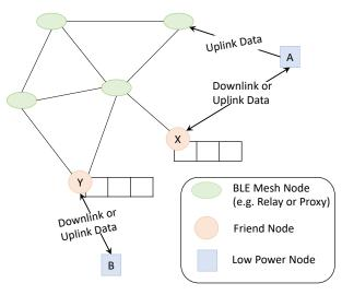
Figure 1. BLE mesh network.
