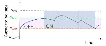
Figure 4. Intermittent behaviour of a batteryless LPN harvesting continuously.
