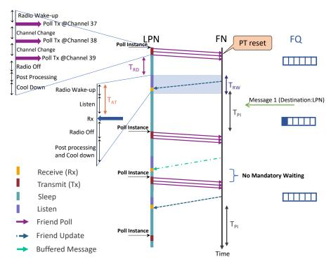
Figure 3. Sequence diagram of the messages exchanged between the LPN and FN to receive DL packets.
