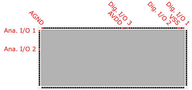
Figure 9 – Die map with measured pins highlighted in red where Dig. I/O stand for a digital input/output pin and Ana. I/O for the analog input/output pin. VSS is the general ground, AVDD is the analog power supply and AGND is the analog ground pin.
