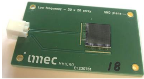
Figure 3: Picture of the PMUT chip, wirebonded to a PCB.
