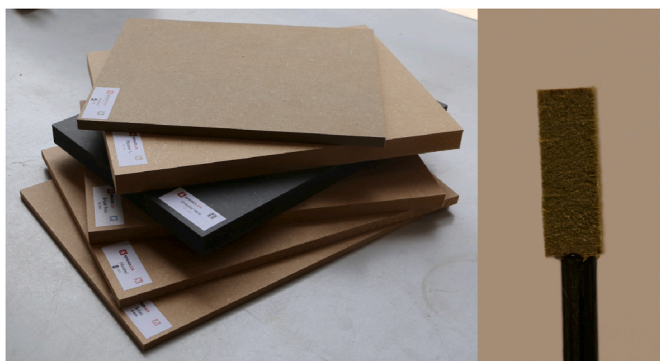
Fig. 1. Left: MDF panel samples of different thicknesses. These are standard line-production panels cut for promotional purposes. Out of such panels, millimetric samples were extracted for X-ray tomography. Right: 2 mm-wide, 9 mm thick MDF sample mounted on a carbon stick for X-ray CT scanning.
