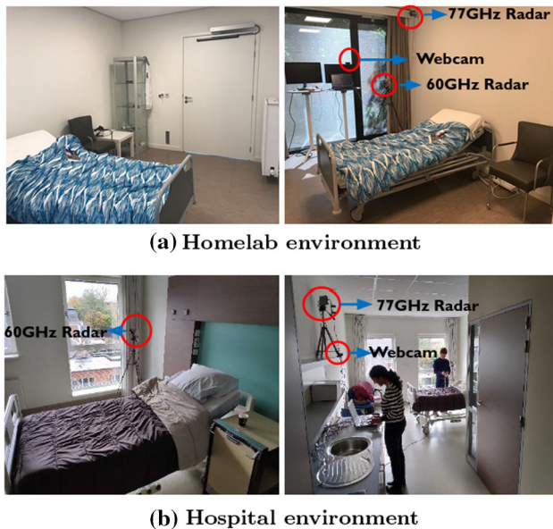
Fig. 5 Data collection: The 77 GHz radar is placed near the ceiling, while the 60 GHz radar and webcam are placed at eye-level height on a tripod
