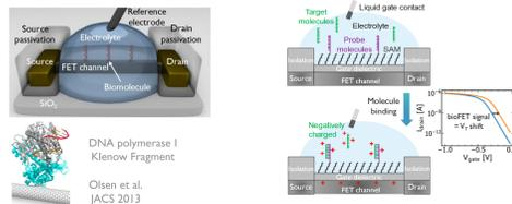
Molecule docks close (1-10nm) to FET surface. Molecule's charge modulates channel charge and FET current
