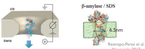
Translocating molecule modulates the recorded ionic current passing through pore
