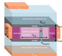
A nanopore wrapped by a nanoscale field-effect transistor (FET). The FET senses single molecules translocating through the pore
