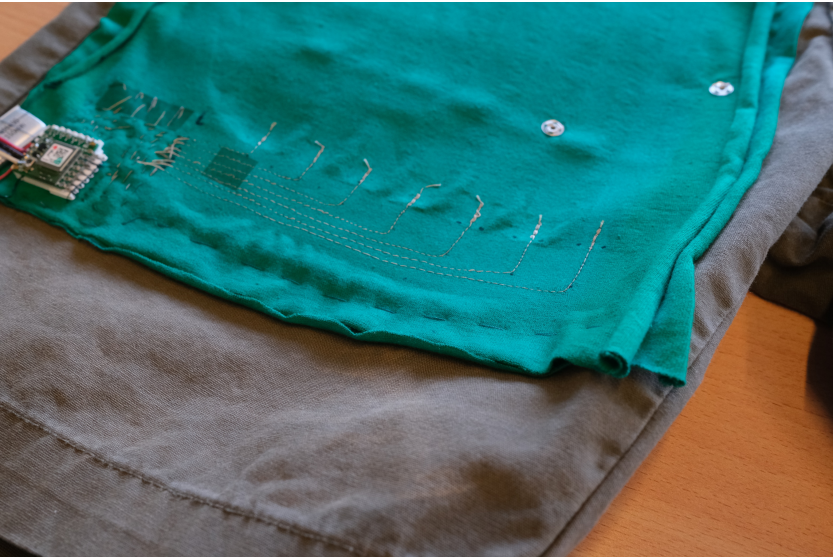
Figure 2.11 Example of a smart textile implementation using a piezoresistive polymer attached inside the fabric.
