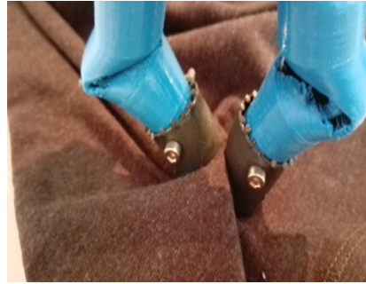
(b) Finger tips with profile to increase friction for grasping.
