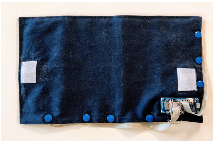
Figure 4.7 Our resulting implementation of a smart textile which is able to detect and translate local forces to a state configuration (for example, folded or unfolded). The smart textile is made using accessible off-the-shelf materials and tools.
