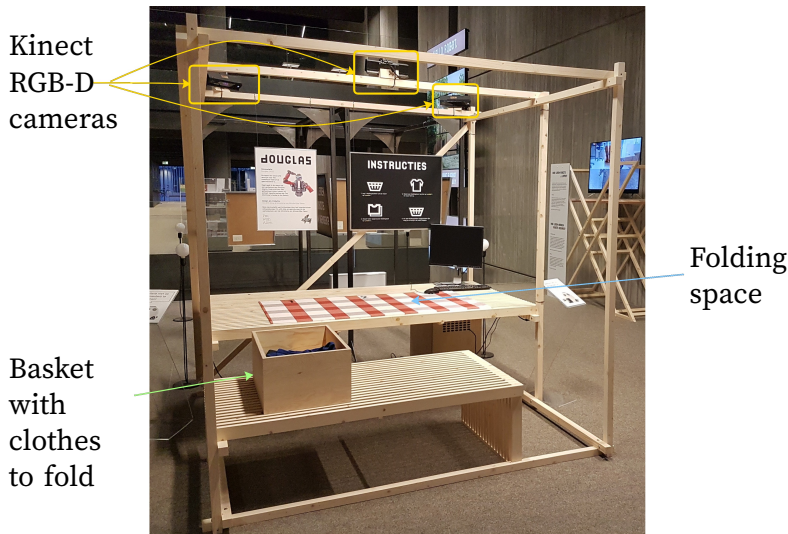
Figure 5.1 Picture of our folding table setup to crowdsource video demonstrations in a public library. There are three Kinect cameras mounted on top of the table that capture the human folding demonstrations. We provide easy and clear instruction to introduce consistency in the demonstrations.
