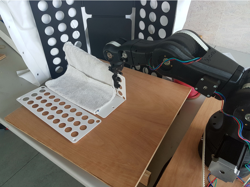
Figure 7.1 First learning to fold a flip-fold can be considered as an instance of curriculum learning towards learning to fold cloth.
