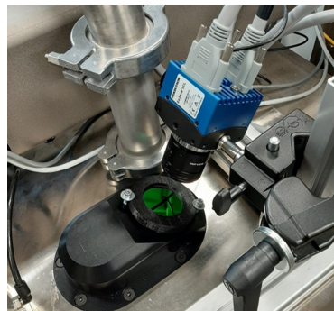
Figure 2. Installation of the high-speed camera on our LPBF printer.
