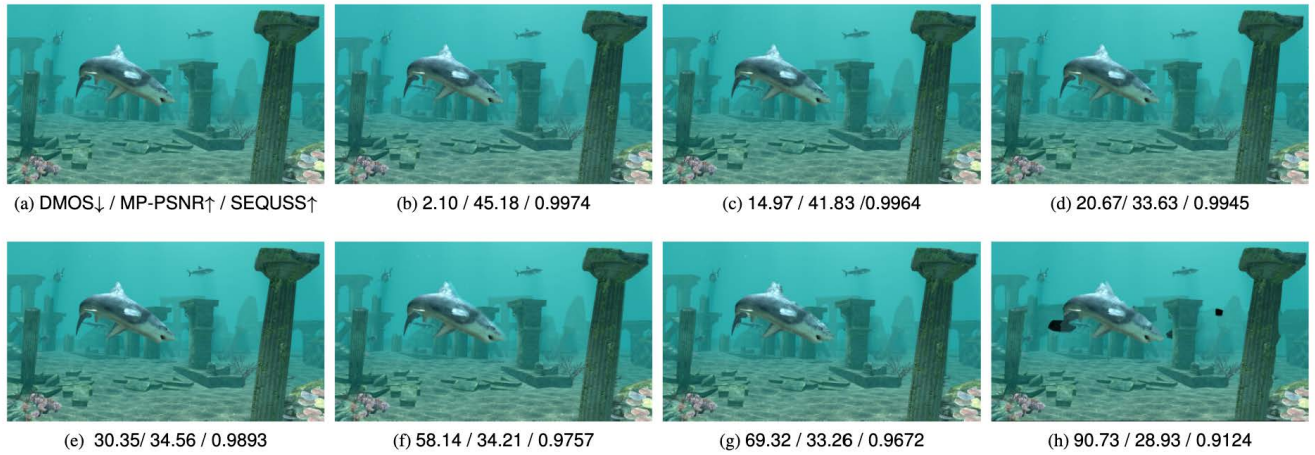
FIGURE 7. Example to visually show the performance of the proposed method. (a) original 'Shark' image from the IETR data set. (b) VRS2, (c) Zhu's, (d) VRS1, (e) Ahn's, (f) HHF, (g) Criminisi, and (h) LDI. The DMOS human opinion scores, MP-PSNR, and SEQUSS scores are presented below each image. The SEQUSS scores (a higher is better \uparrow ) are consistent with the DMOS (a lower value is better \downarrow ).
