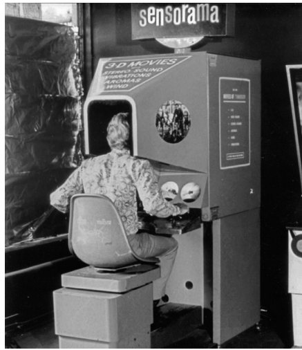
Figure 1.2: The Sensorama, invented by Morton Heilig in 1957, is considered as the first actual device to offer an immersive experience. It was designed to create the sensation of being “in” a movie while watching it.
