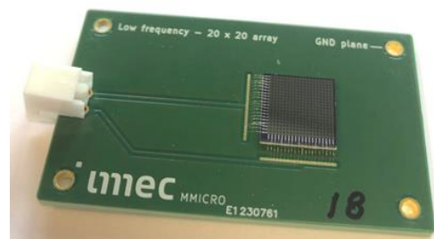
Figure 17: Picture of the PMUT chip, wirebonded to a PCB.
