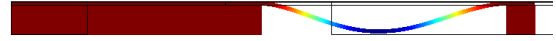
Figure 5: FEM model of a 420 \mu\text{m} membrane donut PMUT with a 300 \mu\text{m} diameter pillar reaching a resonance frequency of 340 kHz.
