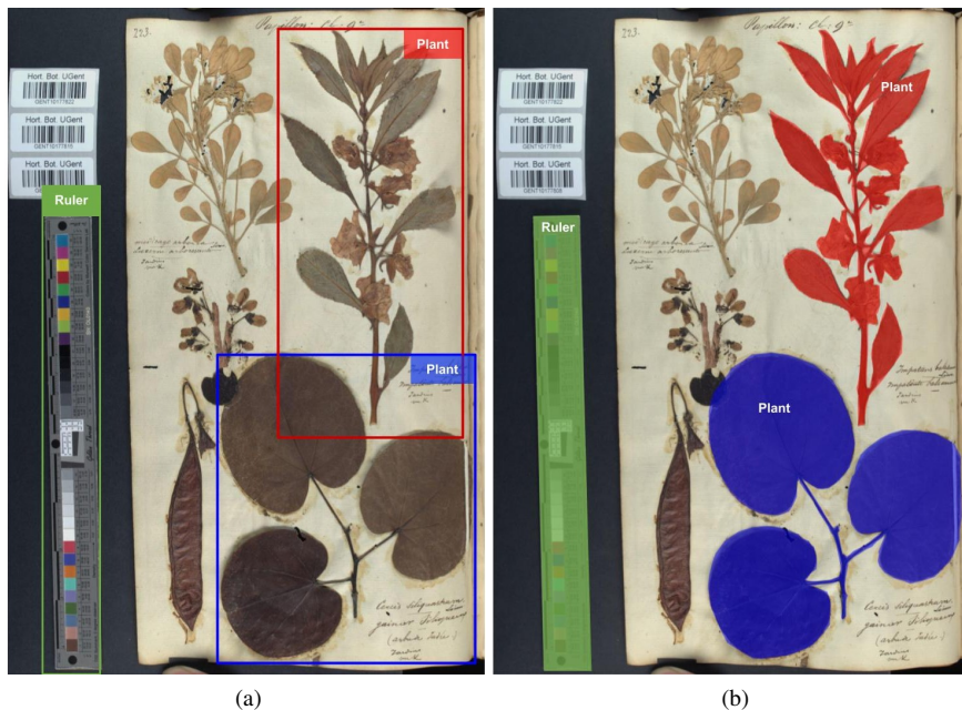
Figure 1.4: An example output produced by (a) an object detection algorithm, and (b) an image segmentation algorithm
