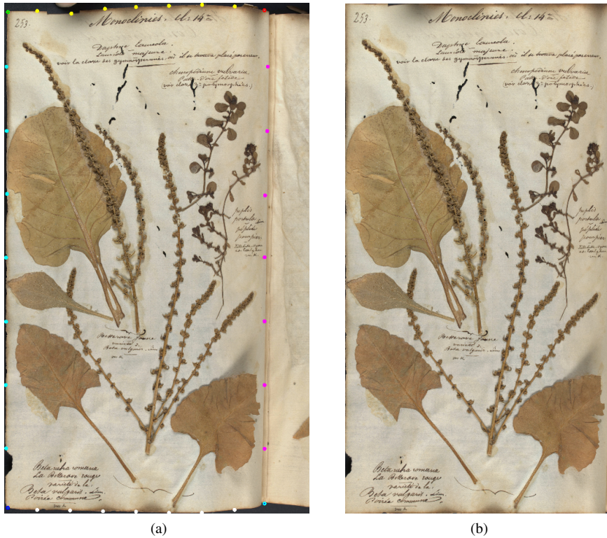
Figure 2.10: An example of morphological correction for flattening the page in order to reduce deformation. (a) is the original image with chosen hull points for flattening and (b) is the subsequent flattened image.
