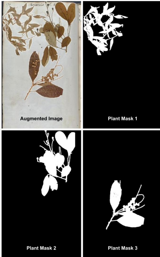
Figure 3.8: Modified version of mosaic augmentation used for training segmentation models. As seen in the image, an augmented image is generated by placing three plant masks on a empty page image.
