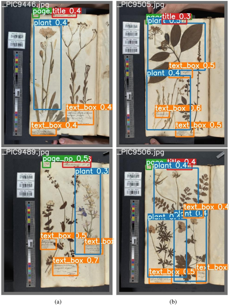
Figure 3.3: Feasibility experiment results of the Yolov3 model trained on 70 labelled herbaria pages. The text regions are well detected whereas the plant boundaries require a lot more training examples to perform as expected.
