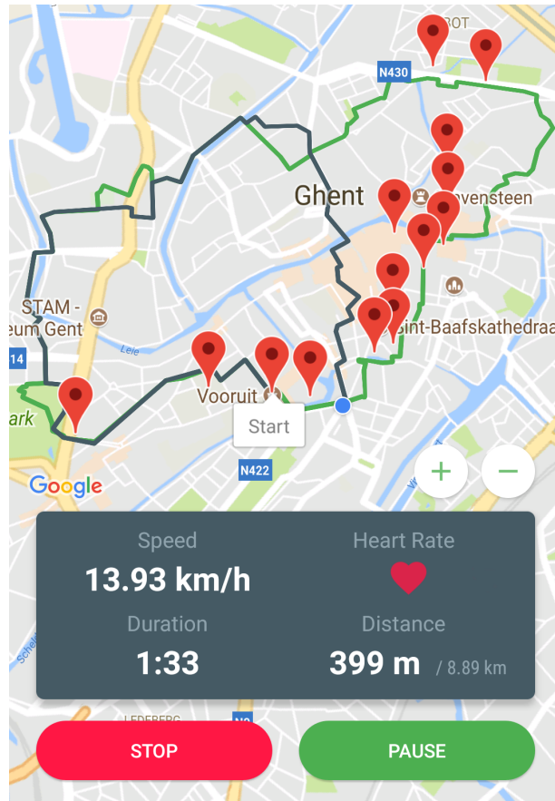
Figure 6.3: Runamic: A Dynamic Route Generation Application. The figure shows an active routing screen of the application. The green line segment in the figure denotes the currently followed route while the blue one denotes a shorter route, requested dynamically.
