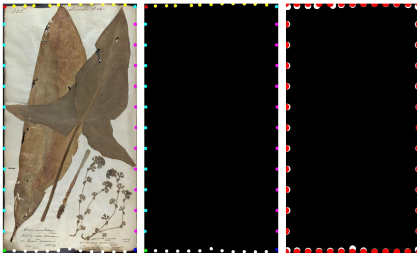
Figure 2.9: Steps involving morphological correction. Based on the page mask, equidistant hull points are chosen along the perimeter of the mask. However, for a flat page, the same points would be a rectangle (red points). Therefore, using the hull points, the entire image is remapped to the expected rectangle.
