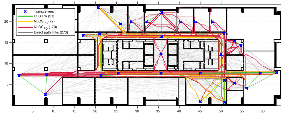
Figure A1. The resulting estimated propagation paths are presented in this figure. The resulting (concatenated) geodesics indicated as paths in green, yellow or red are a result of applying the algorithm in Algorithm 1 to the direct paths indicated as the gray lines.
