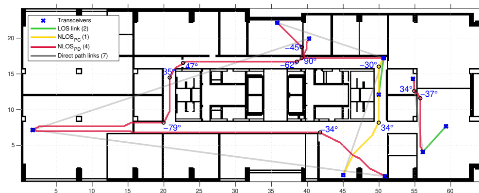
Figure 4. A visualization of the parameters produced by the algorithm, showing direction changes along the geodesic paths expressed in degrees, wall crossings by the direct paths and wall crossings by the geodesic paths. A randomly selected subset (approximately 3% of all links) is generated for visualization.
