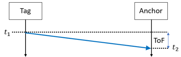
FIGURE 14. ToF localization technique.
