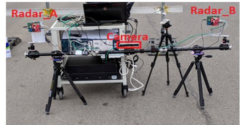
Fig. 5. Overall system and set up for outdoor measurement.
