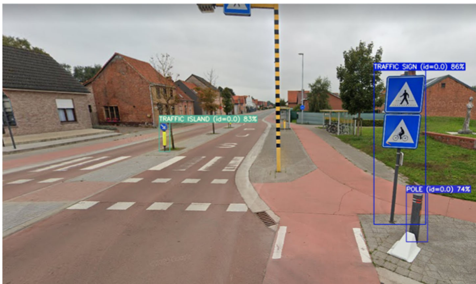
Fig. 11 Example of a street scene with the detected traffic infrastructure objects. The left, yellow traffic island pole is commonly used in Belgium and the Netherlands to signal traffic islands
