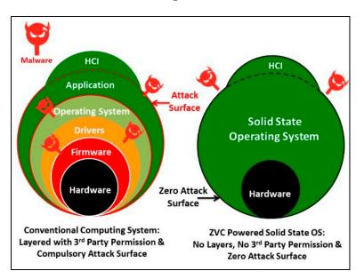
**Figure 15.** Diagrammatic illustration of the conventional multi-layered computer architecture in comparison to the projected compact zero attack surface design of ZVC.
