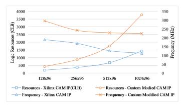
**Figure 4:** Operating frequency and resource utilization of the CAM directly implemented with the Xilinx tools (referred to as Xilinx CAM IP) and the speed-optimized CAM architecture (Custom Modified CAM IP)
