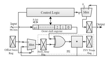
Figure 6: FNV-1a - serialized hardware architecture block diagram
