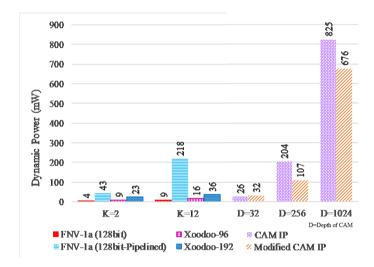
Figure 14: Dynamic Power Consumption of Bloom-1 (Using FNV & Xoodoo-NC), and CAM
