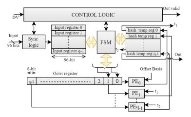
Figure 7: FNV-1a - Pipelined hardware architecture block diagram
