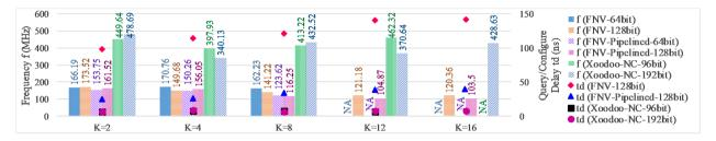
Figure 13: Maximum Operating Frequency and Delay of Bloom-1
