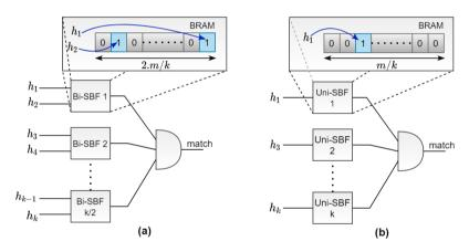
Figure 3: Parallel Bloom filter logic (a) using Bi-SBF and (b) using Uni-SBF
