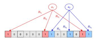
Figure 1: Standard Bloom filter (SBF) representation
