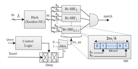
Figure 11: Parallel Bloom Filter hardware architecture
