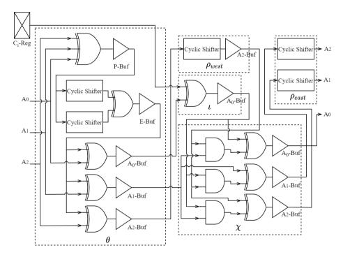
Figure 9: Xoodoo-NC Round, which is implemented 2 or 3 times in combinational logic for a 96-bit or 192-bit hash output, respectively.
