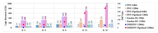
Figure 12: Resource Utilization of Bloom-1: Logic resources and DSP units
