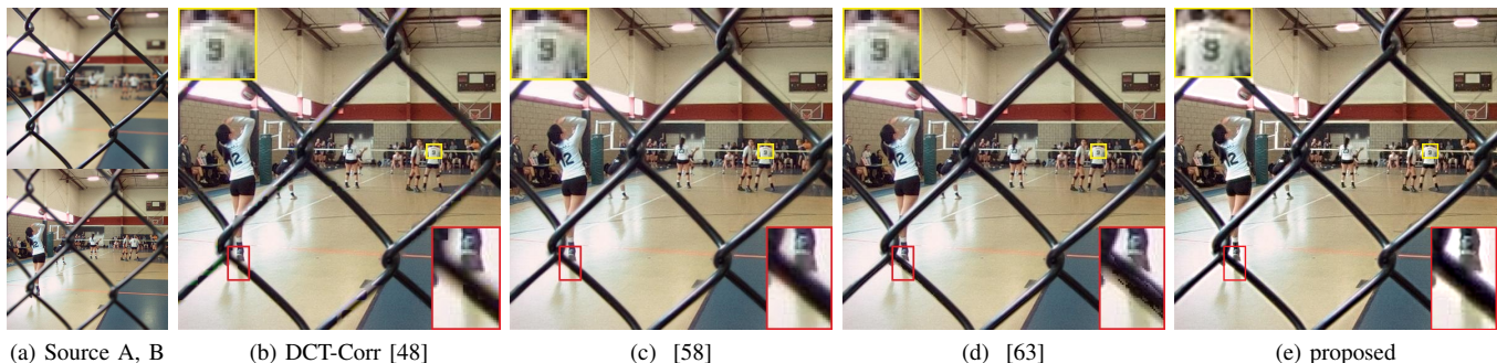
Fig. 7. A multi-focus image fusion example. The proposed model in (e) is compared against a transform-domain method in (b), and two CNN designs in (c), (d). The proposed design generates a sharper all-in-focus image with no visible artifacts around edges, resulting in a more natural output.
