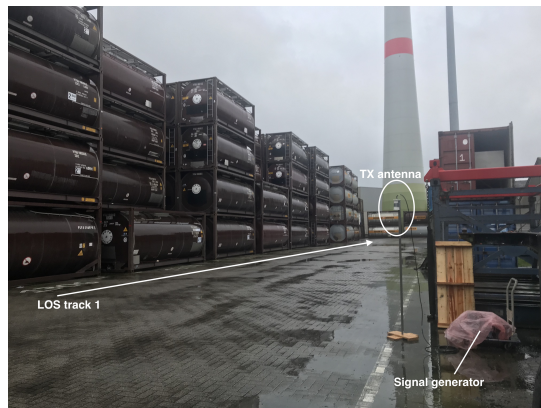
(a) TX antenna and Line-of-Sight track 1
