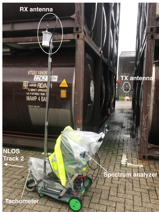
(b) Mobile cart with RX antenna and spectrum analyzer
