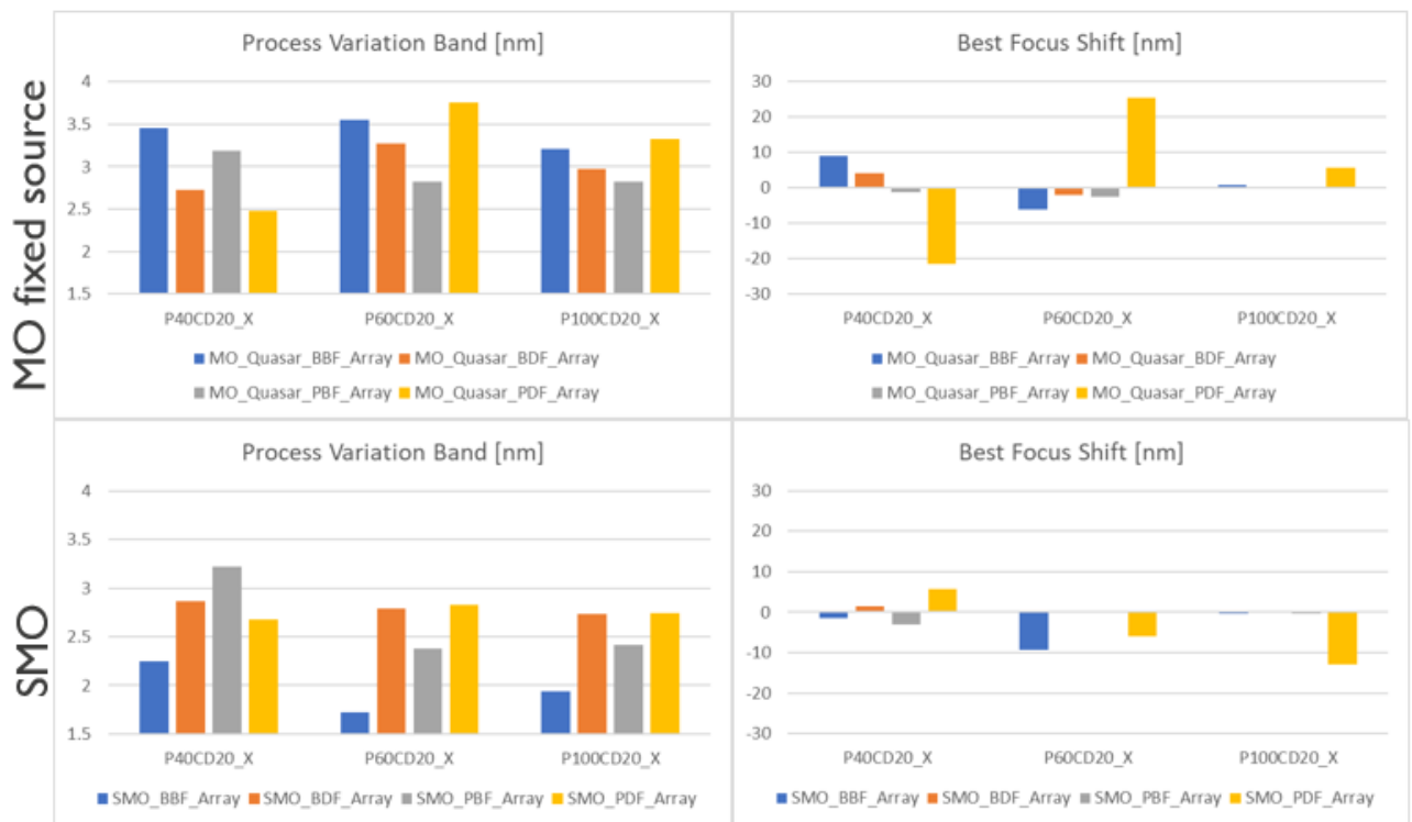
Figure 6. Histogram plot of PV Band (process variation band), best focus shift at CD20 X cutlines of pitch 40, 60 and 100nm. (Orange - reference BDF, blue BBF, grey PBF, yellow PDF)
