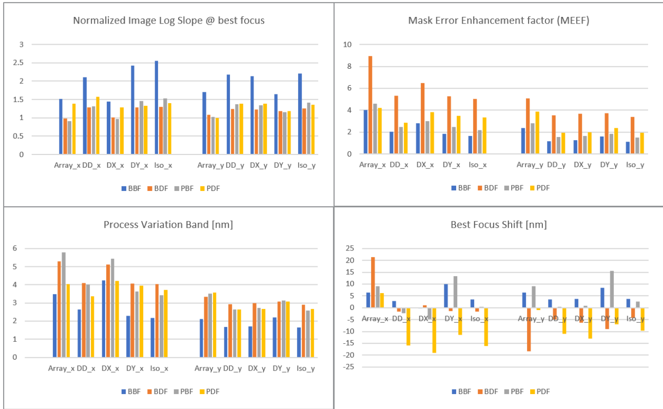
Figure 10. Histogram plots of NILS at best focus, MEEF, PV Band (process variation band), Best focus shift at pitch x 42nm pitch y 36nm designs: array, iso, doublet X (DX), doublet Y (DY), and doublet diagonal (DD) (Orange - reference BDF, blue BBF, grey PBF, yellow PDF)
