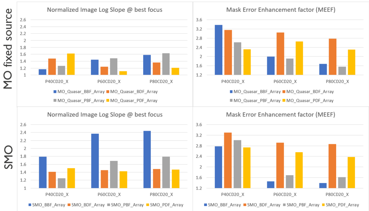
Figure 5. Histogram plot of NILS at best focus and MEEF at CD20 X cutlines of pitch 40, 60 and 100nm. (Orange - reference BDF, blue BBF, grey PBF, yellow PDF)
