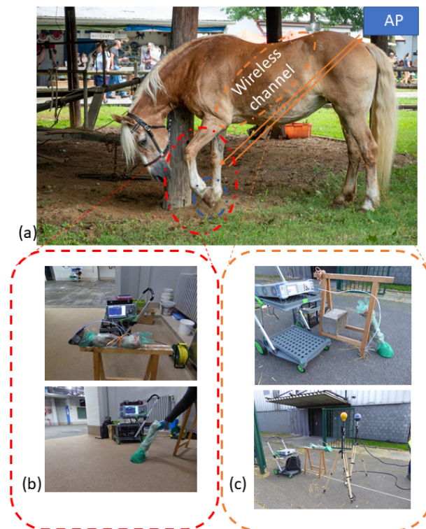
Figure 3. (a) the overall concept of the project; a mobile sensor embedded in the horseshoe communicating the behavioral data of the horse to a access point located somewhere in the pasture the horse resides. This work studies the combined antenna–channel modeling of this situation; (b) shows the constructed pad, the severed horse leg, covered in a hygienic veterinary glove; part of the hoof is uncovered by the glove and the hoof pad is attached to it with tape. The top picture is the air-case setup. The iron is attached by means of the green tape as seen on the ground-case setup, the bottom picture; (c) the path loss measurement setups as discussed in Section 4.1.
