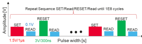
Fig.11 Schematic for LRS and HRS endurance test up to 1\text{E}8 cycles.
