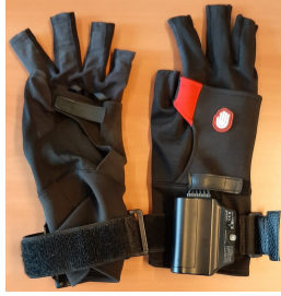
Figure 2: The Noitom Hi5 VR haptic gloves.
